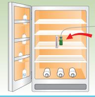
Place the probe of the digital thermometer in the center of the refrigerator.
