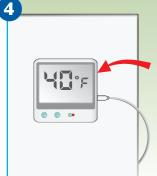
Attach the display of the digital thermometer to the outside of refrigerator, either on the door or on the side.
